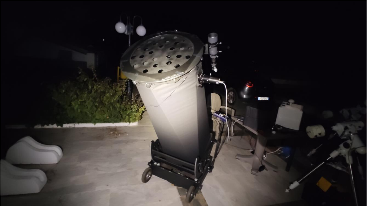
Noschese's masked "Leviatan" 50 cm Newton Dobson-mount telescope, with the mask.
